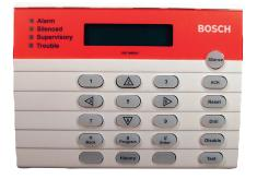
The FMR-7033 LCD Keypad combines remote annunciator and controller functions for fire alarm systems controlled by the FPD-7024 Fire Alarm Control Panel (FACP). It operates identically to the user interface on the FPD-7024 FACP. You can connect up to four FMR-7033 keypads to an FPD-7024.
